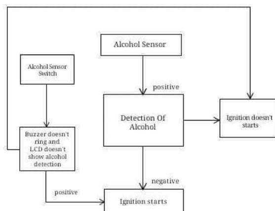
Fig.2 Flowchart of working of system
